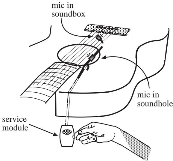
**Step 3** Attach the service module to the strap button attachment and plug the mono guitar cable (2 conductor) into the output jack. Remember to use the 1/4"-XLR adapter for P.A. boards and acoustic amps.
